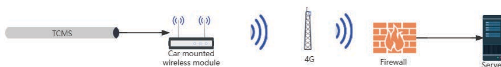
Figure 1. Vehicle analysis system data link
